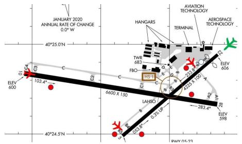
*Note*. The image is of a hypothetical SAFE-RWSL installation at the Purdue University airport (limited tower operations). The red circles indicate a red indication on a DAL/REL at a given location. The red airplanes show aircraft in position given a stop indication, and the green airplane shows the approaching aircraft. Airport diagram adapted from "FAA Airport Diagrams" by Federal Aviation Administration, 2022
