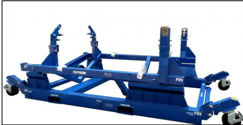
Figure 6. An Electric Dolly for Engines, Similar to That to be Used in Battery [19].
