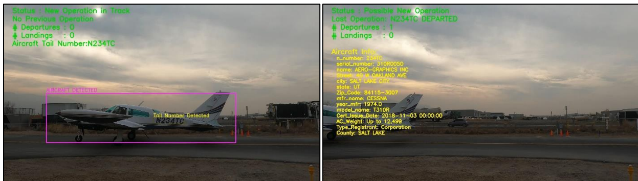
Figure 13. AIVATS software performance during (left image) and right after (right image) the aircraft operation in layout 2
