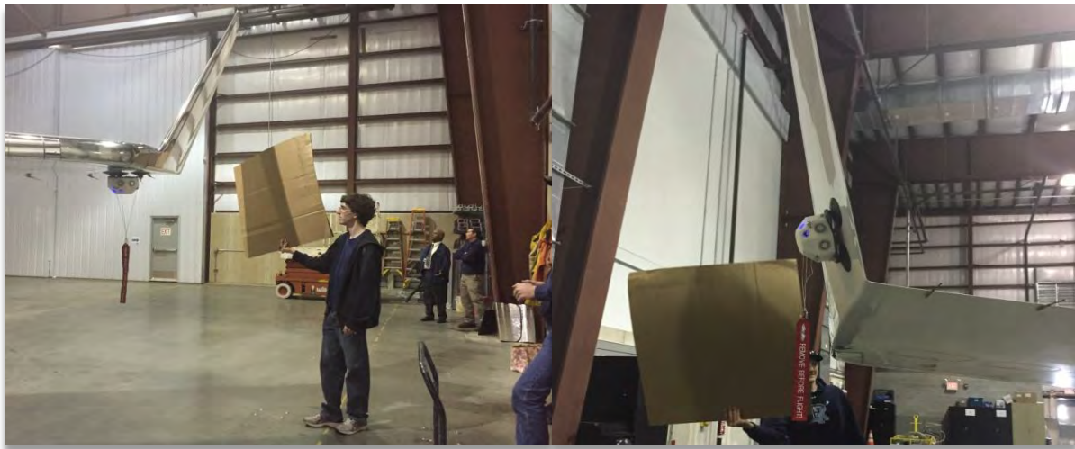
Figure 15: Testing the detection of a board while the Wingman 360 is attached to an aircraft
