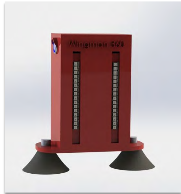
Figure 21: Receiver module box with LEDs and buzzer
