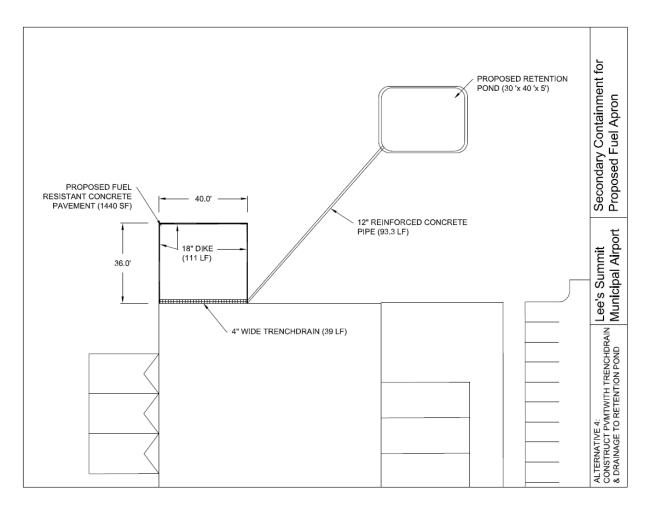
Figure G.4. Proposed Mobile Refueler Parking Area Design: Alternative 4
