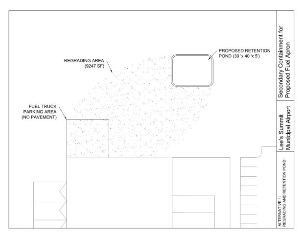
Figure G.1. Proposed Mobile Refueler Parking Area Design: Alternative 1
