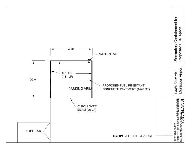
Figure G.2. Proposed Mobile Refueler Parking Area Design: Alternative 2
