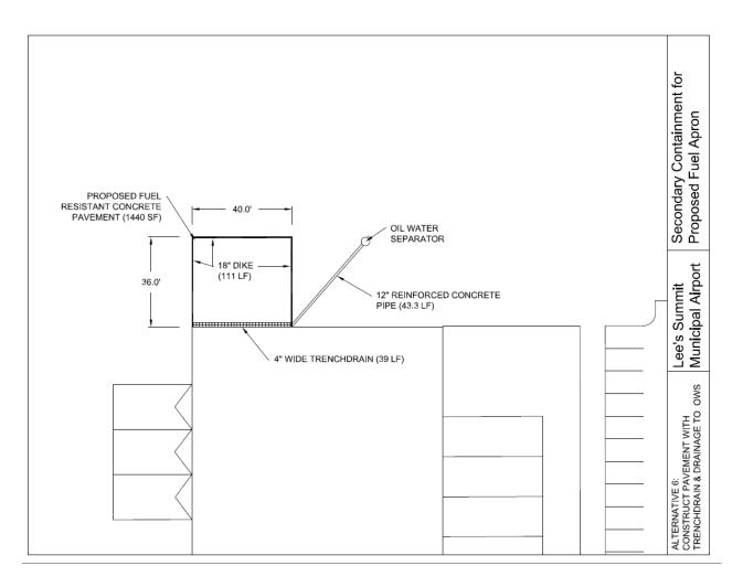
Figure G.6. Proposed Mobile Refueler Parking Area Design: Alternative 6
