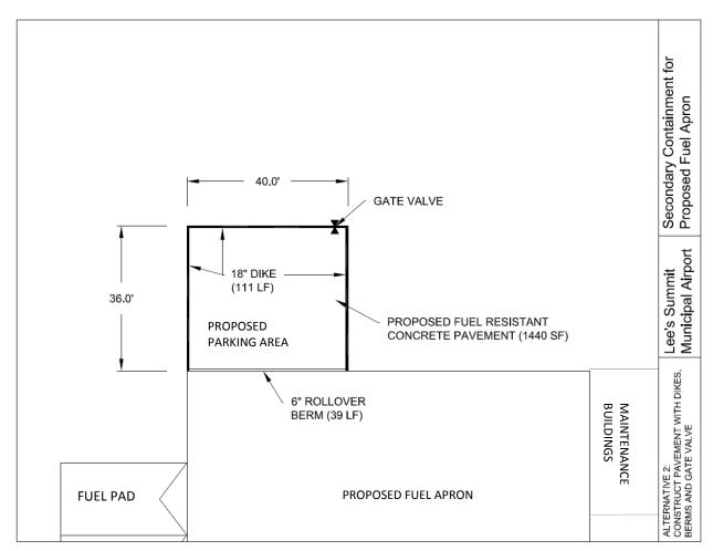
Figure 5.1. Proposed Mobile Refueler Parking Area Design: Alternative 2
