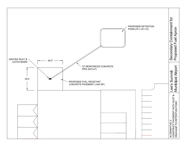
Figure G.3. Proposed Mobile Refueler Parking Area Design: Alternative 3
