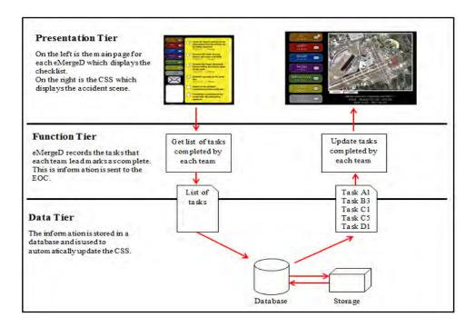
Figure 1. Information Transfer between the CSS and the Tablet Devices
