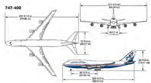
Figure 4: Overall aircraft dimensions of Boeing 747-400 showing the height limitations for snow prevention structures (Boeing).
