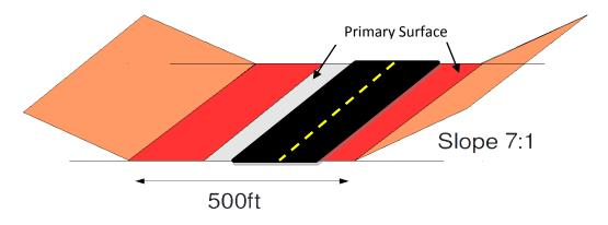
Figure 1: Illustration of Primary Surface Limitations
