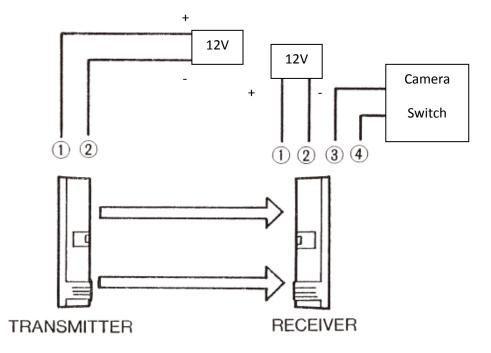
Figure 13: Sensor Wiring Diagram
