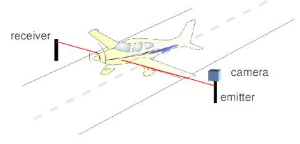
Figure 2: Photoelectric Beam Sensor System
