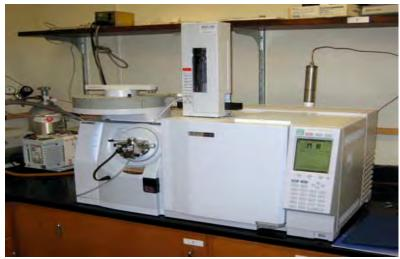
Figure 6. Gas Chromatograph-Mass Spectrometer
