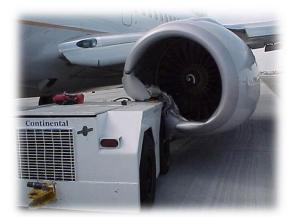
Figure 5: Collision between GSE and aircraft
