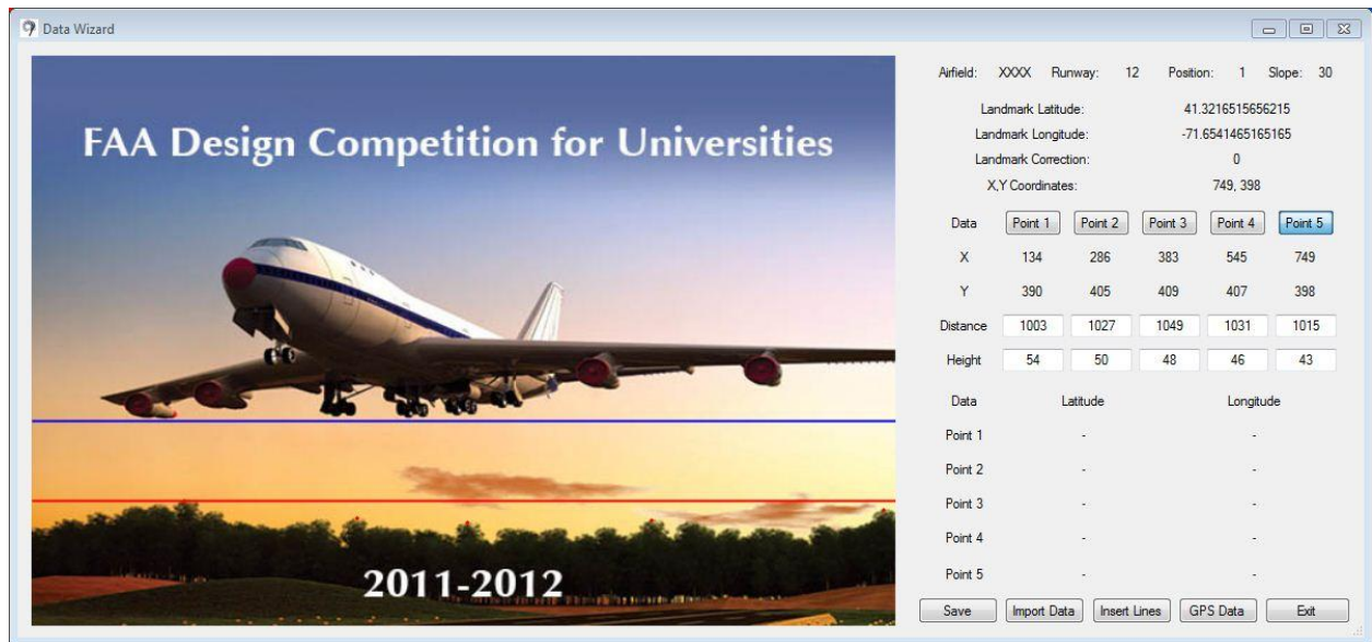
Figure 9: Data Wizard complete with selected data points, distance and height measurements, controlling obstruction line, and current approach slop line.
