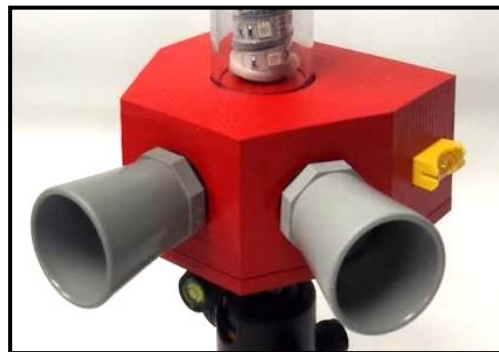
Figure 11: Circuit and sensor housing.
