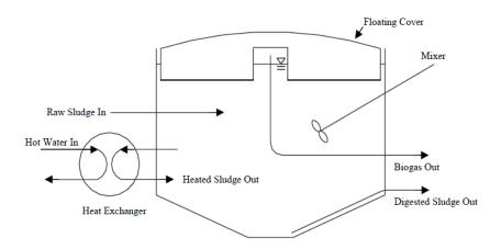
Figure 5. Anaerobic Biogas Reactor
