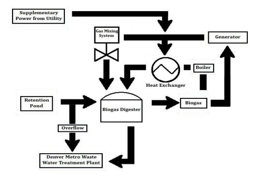
Figure 11. Flowchart Depicting Biogas Digester System
