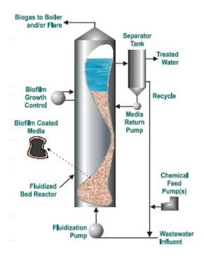
Figure 6. Anaerobic Fluidized Bed Reactor
