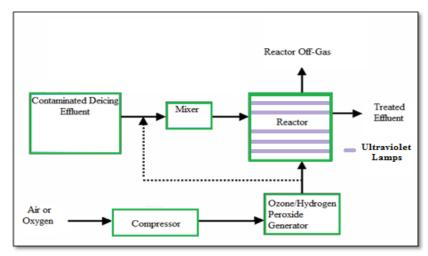
Figure 7. Illustration of Ultraviolet Degredation Coupled with Oxidizing Compound
