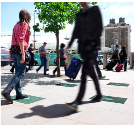
Figure 7 – Pavegen tiles capture energy from footsteps [30]
