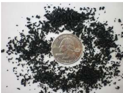
Figure 11 Crumb rubber size in comparison to a quarter (DeerPath Recyclers, 2014)
