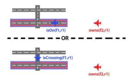
Returning to our example, the arriving plane has received the crossRunway message with the value "Two Four Left." This fires the "isOn" rule for this airplane. The departing plane has received the clearedForTakeoff message with the runway "Two Four Left." and the "owns" rule fires. Once this assertion is added the knowledge base, the "incursingOn" rule fires and both airplanes receive the predicate "incursingOn" with the object "Two Four Left" in the knowledge base.
