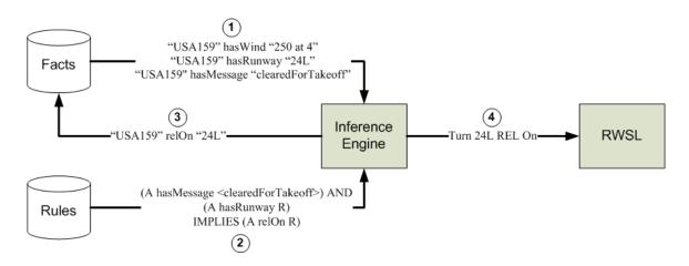
The rule states that if there is an airplane that has received a "clearedForTakeoff" message and this same plane is associated with a runway, then the RWSL system should be turned on for the given runway. Due to the existence of the hasMessage and hasRunway assertions about flight "US Air one five nine," a new statement regarding REL illumination is added to the knowledge base.
