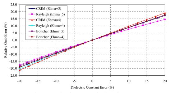
Figure 7. Relative  $G_{mb}$  error as a function of  $\varepsilon_{HMA}$  error.
