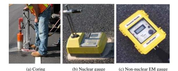
Figure 1. Available methods for density measurements for HMA airport pavements.
