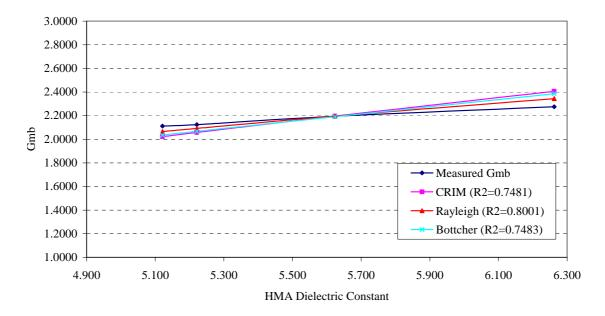
Figure 11. Measured and fitted  $G_{mb}$  variation as a function of  $\mathcal{E}_{HMA..}$
