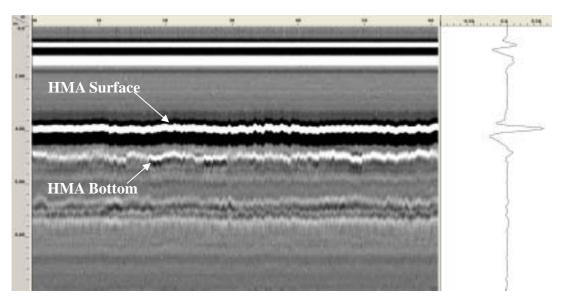
Figure 13. GPR image from the composite pavement with HMA surface.
