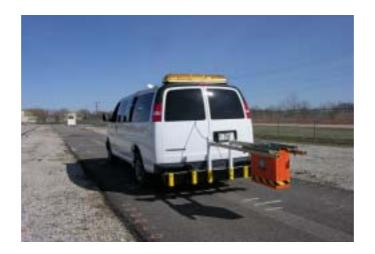
Figure 12. HMA pavement survey using a 2.0GHz air-coupled antenna.
