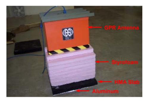
Figure 9. GPR data collection from the slabs.
