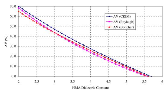
Figure 6. Air voids variations as a function of  $\varepsilon_{HMA}$ .
