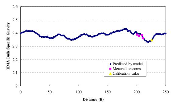
Figure 14. Bulk specific gravity profile of the HMA surface.
