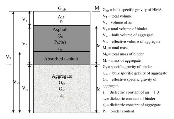
Figure 4. HMA volume and mass composition.
