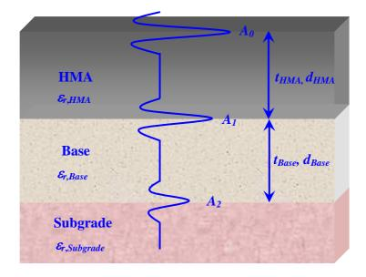
Figure 3. Typical GPR signal for an HMA pavement system.
