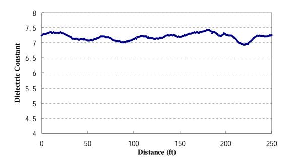
Figure 14. Dielectric constant profile of the HMA surface.
