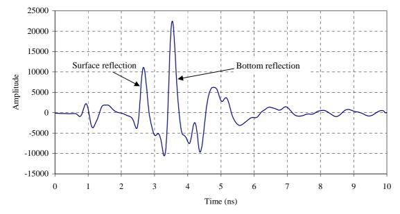
Figure 10. Typical GPR scan collected on a HMA slab.
