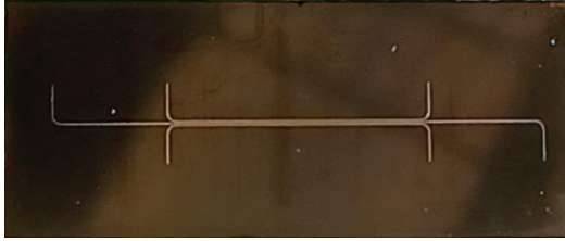
Figure 3: Three microstrips on an AlON substrate, two U wires and a central Z wire. These microstrips used deposited Ag with adhesion layers of Cr and Ti.
