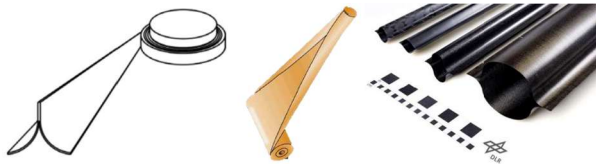
Figure 2. Deployable boom types: TRAC (left), STEM (middle), CTM/lenticular (right) [7].
