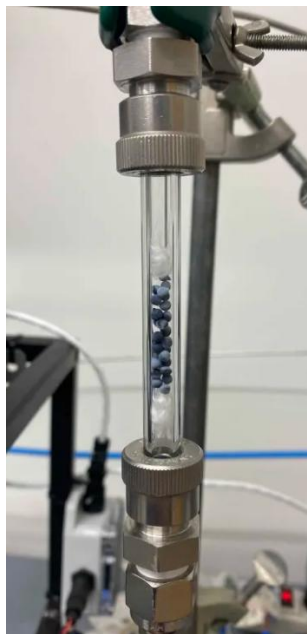
Figure 8. Image of sorption column with aerogel sorbent placed inside before the addition of the thermocouple and heating tape. Image from Daniel Lobree.
