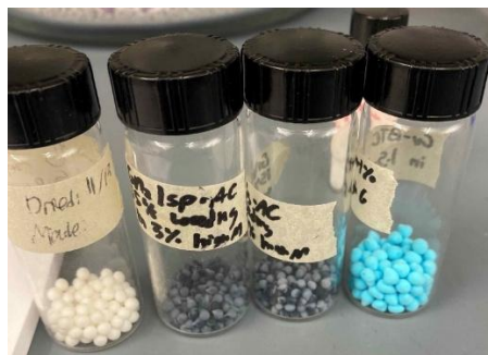
Figure 7. Image of synthesized 15wt% \text{Gn}_2\text{CO}_3 -AC and 15wt% \text{Gn}_2\text{Isp} -AC aerogels. Image from Daniel Lobree.
