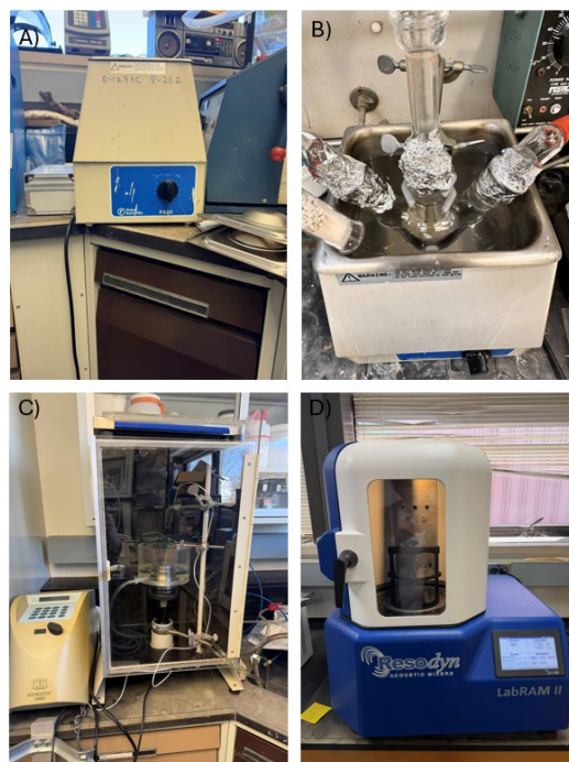
Figure 2: Various equipment used for dispersion experiments: A) bath sonicator, B) three-neck flask setup for in-situ polymerization, C) cup horn sonicator, D) acoustic mixer
