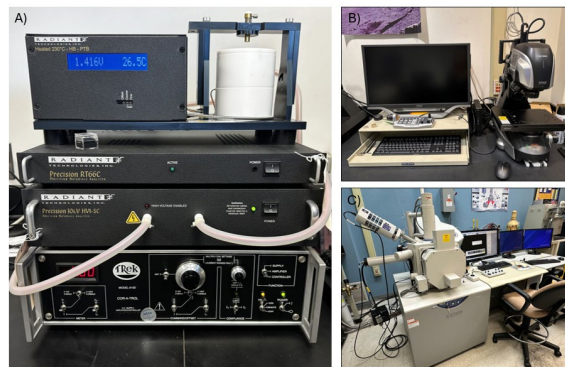
Figure 4: A) Ferroelectric testing equipment, B) optical microscope, and C) SEM testing equipment
