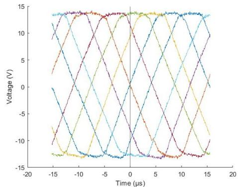
Figure F: Voltage Waveforms from Function Generator with Eight Symmetrical Phase Shifts
