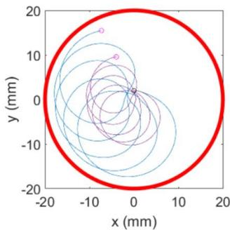
Figure B: Trajectory of Nitrogen Ion at 35kHz (Blue) and 77kHz (Purple)
