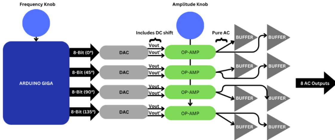
Figure C: Signal Routing Diagram
