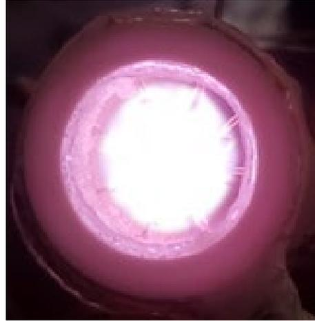
*Figure G: Helium Plasma Observed in Gas Tube Electrode*
