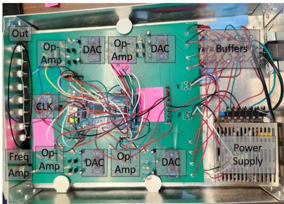
Figure D: Function Generator
