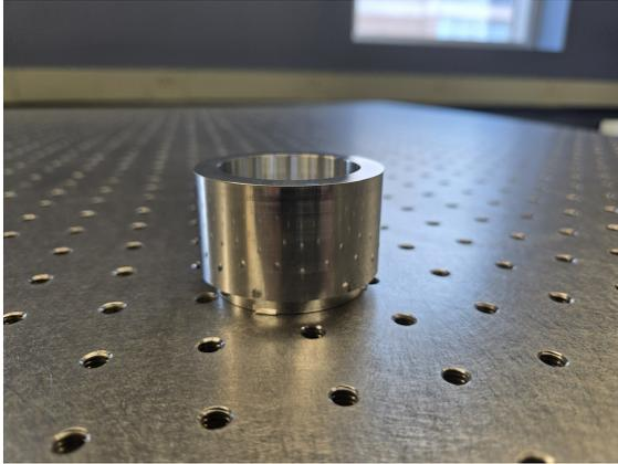
Figure 5: The coupling device fits onto the sample chamber at the bottom and has a 2.2in outer diameter made to match with a 2in lens tube, allowing for coupling via a coupling sleeve. This design allows semi-rigid connection while maintaining rotational freedom, permitting the design and layout of the experiment to change in future projects.
