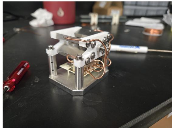
Figure 7: Sample configuration of ion trap connected to the rf-board seated beneath.
