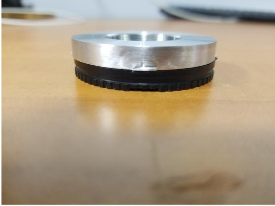
Figure 2: Direct comparison between newly designed window modifiers (silver) and original window covers (black).
