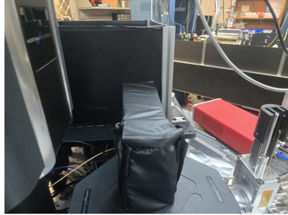
Figure 4: A periscopic mirror sits above the lid window of the sample chamber, sending light into the sensor box.
