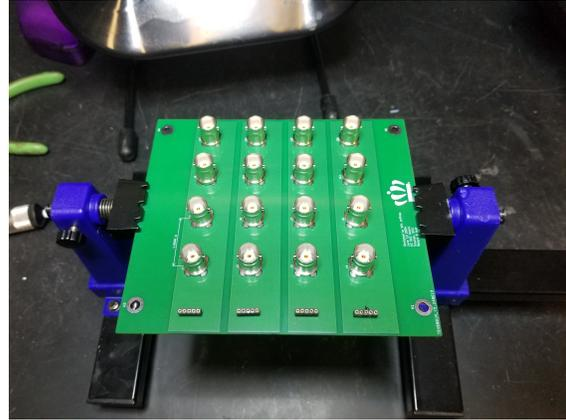
Figure 6: Four-by-four BNC array board for connecting DC and low-frequency AC signals to the interior of the sample chamber.
