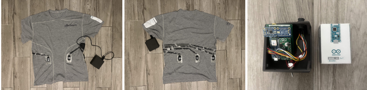
Figure 1: Triton Systems vibrotactile garment front and Arduino nano 33 IOT board.
