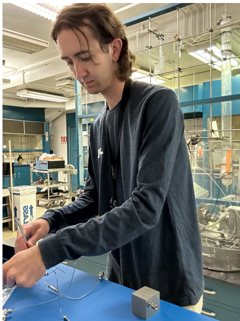
Figure 2. Setting up the titanium 3D-printed PLOT column into the system with the TCD for sample injection analysis.
