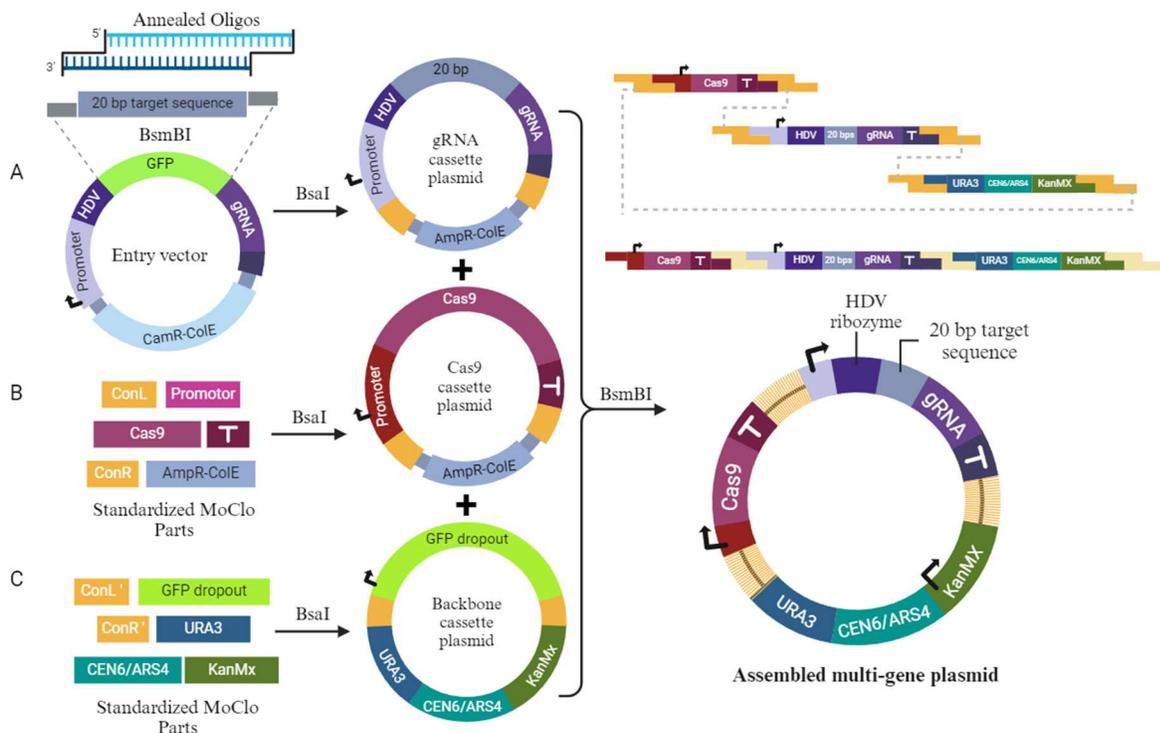
Figure 4. Specialized Modular Cloning workflow to produce Multi-gene Plasmid
