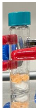
Reaction to form the solid-supported oxoammonium salt
