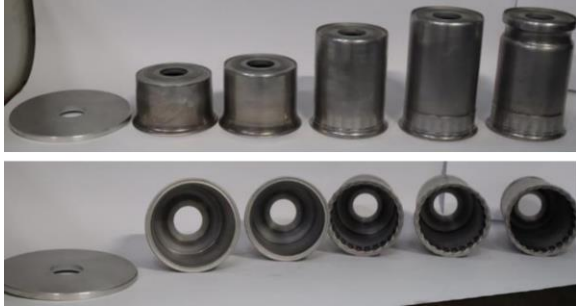
Figure 3. Top and side views of the incremental forming steps using the VUD 600 standard protocol.
