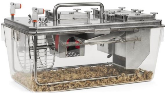
Figure 2. Promethion cage layout with the feeding hopper (front right), water hopper (back right), and mass hopper with red-shaded frames (center). This is a stock photo provided by Sable Systems International which includes an exercise wheel (far left) that was not used in this experiment 15 .
