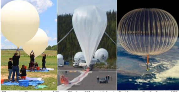
Figure 1: Examples of Free-Flying High-Altitude Balloons (Left: Latex [8], Middle: Zero-Pressure[19], Right: Super-Pressure [18])
