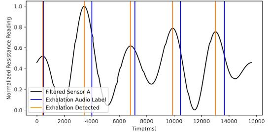
(b) Filtered Sensor A Data With Peak Detection
