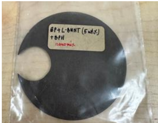
Figure 1: Example of a bulk composite epoxy disk with 5 wt% BNNTs. Sample was rough cut with a bandsaw and then polished to a uniform diameter of 12.5mm by a lathe.
