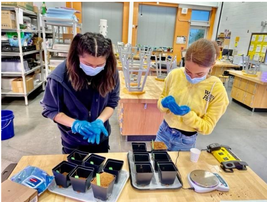
Photo 1 Caption: This Plant the Moon Challenge team grew radishes in lunar highland simulant in their high school science lab and varied the light source lumens and nutrient amendments in their experimental design.
