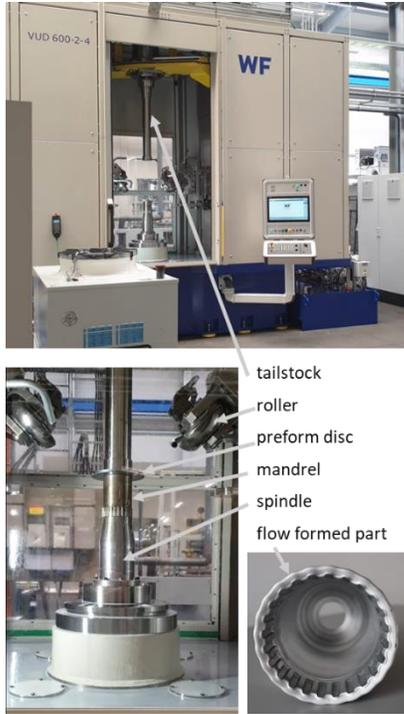
Figure 1: WF VUD-600 vertical flow forming machine with main components labeled.
