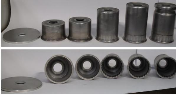
Figure 2: Conversion of a disc-shaped preform to a demonstration part through: spin forming, forward flow forming and gear tooth formation, reverse flow forming, and hub forming.
