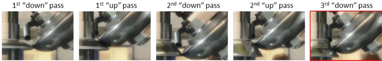
Figure 8: Image series showing the progressive spin forming steps for Al 6061. The final image shows the point of failure for alloys 2139 and 5083.
