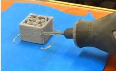
**Figure 4.** Initial cutting tests maximizing the shear force between substrate and printed part.
