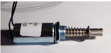
Figure 2: Solenoid for MSBS testing.
