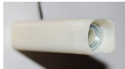
Figure 4: Solenoid housing with Solenoid base inside for MSBS testing.
