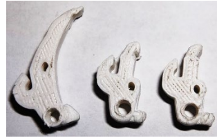
Figure 6: 3D printed Long Gripper and Short Grippers for MSBS testing.
