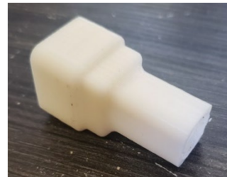
Figure 3: Cap for Solenoid Housing for MSBS testing.
