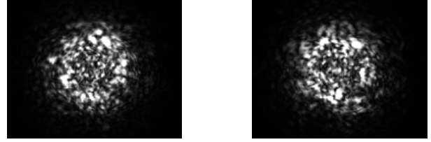
Figure 2: A comparison of the multimode fiber output “speckle” patterns for 0^\circ (left) and 45^\circ (right) polarization angles.
