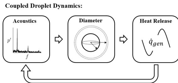
*Figure 1: The coupling between acoustic waves, droplet size and heat release provides a potential feedback path for an instability to grow.*
