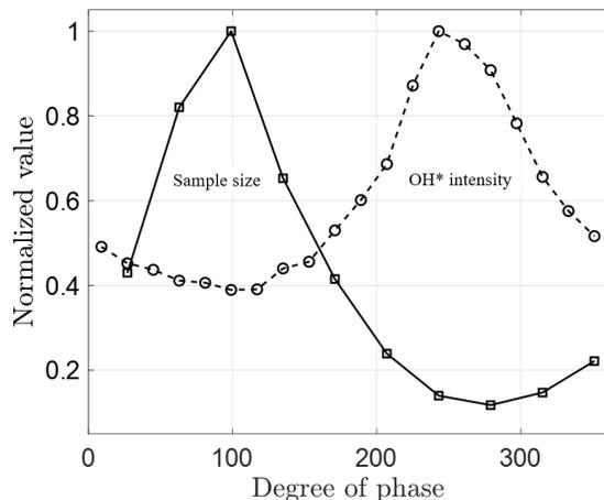
Figure 8: Sample size was found to be out of phase with the OH\* intensity.
