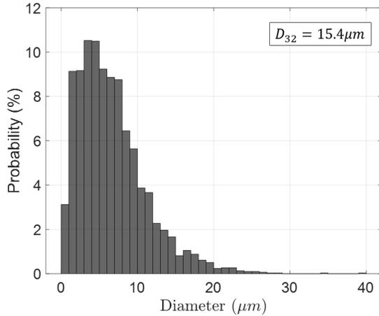
Figure 5: The droplet distribution collected by the PDPA showed a typical distribution for a pressure atomizing nozzle.
