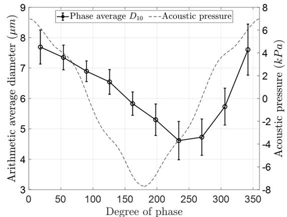
Figure 7: Phase locked droplet diameters show a clear and significant coupling.
