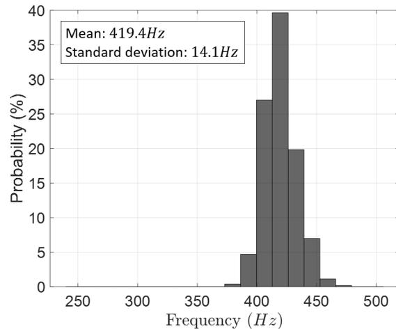
Figure 4: The distribution of instability frequency during a single run show that the instability frequency fluctuated at the quasi-steady state.
