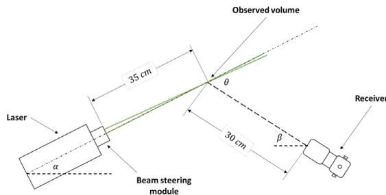
Figure 3: Optical layout of a PDPA system.
