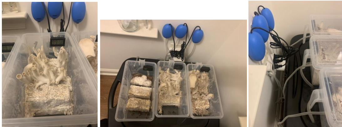
Figure 2: Fully Assembled system. In the center photo, from left to right, is the NFT, Ebb/Flow, and COTS systems. The lid is off in these photos better show the insides of the system.
