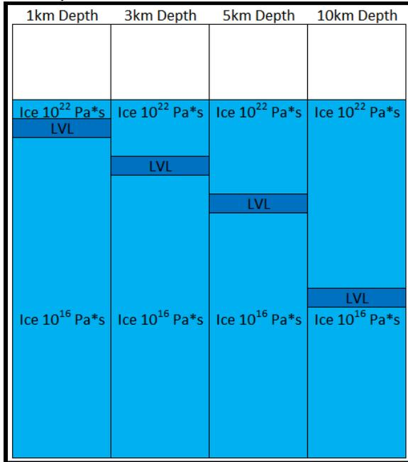
Figure 1: Cross sections of the model setup to scale. The entire ice shell is 19 km thick. The ice above the LVL has a viscosity of  $10^{22}$  Pa\*s. The LVL's viscosity varies as in table 1, with 0 Pa\*s being liquid water. The 1km thick LVL was embedded in the ice at the depths listed in Table 1. The ice below the LVL has a viscosity of  $10^{16}$  Pa\*s.
