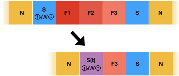
Figure 3: Illustration of the typical spin-triplet JMRAM setup (top) and my proposal to use the newly-discovered equal-spin superconductor  $UTe_2$  (bottom).
