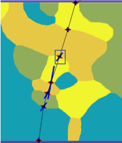
Figure 4: Example of light ray raveling through a completed phase field simulation with the tangent line to the interface (red) and normal (blue) shown. The square shows the location of interest for figure 5.
