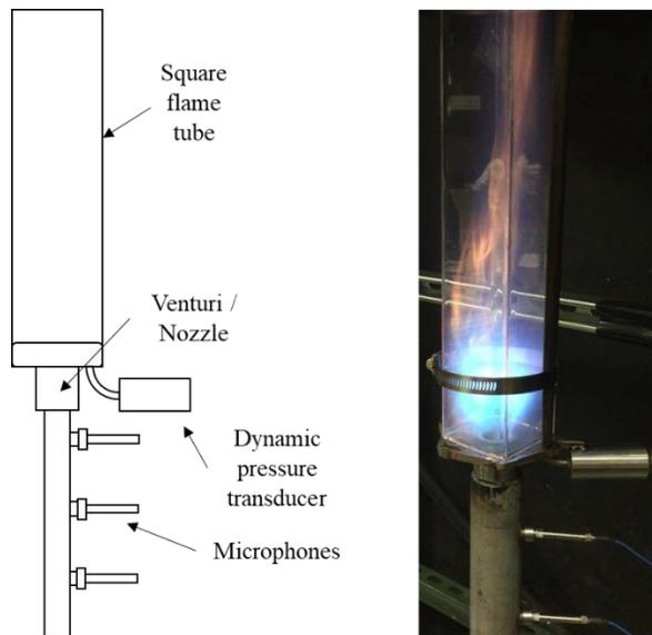
Figure 2: LDI Combustion rig running in a stable mode of operation.
