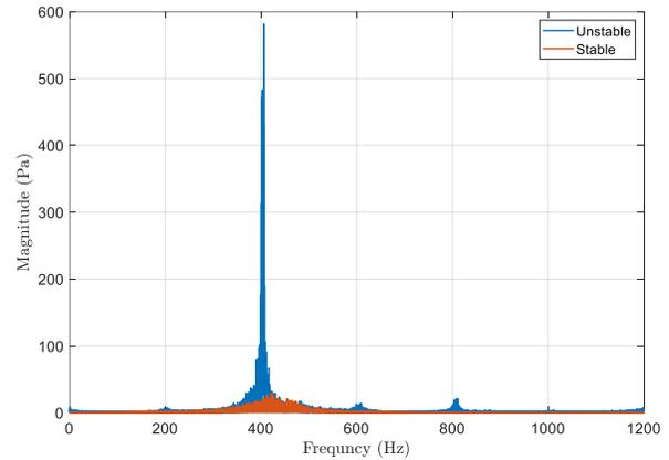
Figure 4: FFT of the dynamic pressure transducer signal in the combustor during the instability in comparison to a stable case. While some 400 Hz excitation was observed, it was far less than during stable operation.
