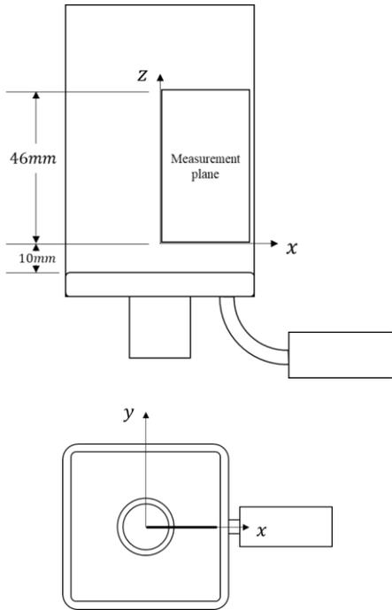
Figure 3: Schematic of the measurement locations. A total of 35 points were targeted.
