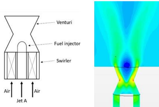
*Figure 1: (Left) The sketch of the LDI injector illustrates key components of the system such as short mixing length. (Right) The axial velocity contour shows the recirculation region anchored to the outlet. This recirculation zone provides the rapid fuel / air mixing which is desirable in lean combustion systems.*
