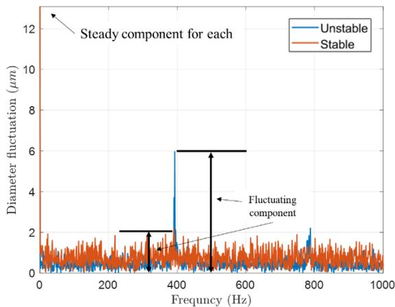
Figure 6: Spectral plot of the diameter signal measured above the dump plane. Definitive
