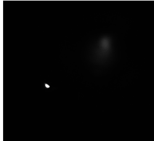
Fig. 11 (top) Focused electron beam spot displayed upon phosphorus screen in dark room. Slight aberration within the center created by femtosecond laser. (bottom) electron beam spot displayed upon mm scale.
