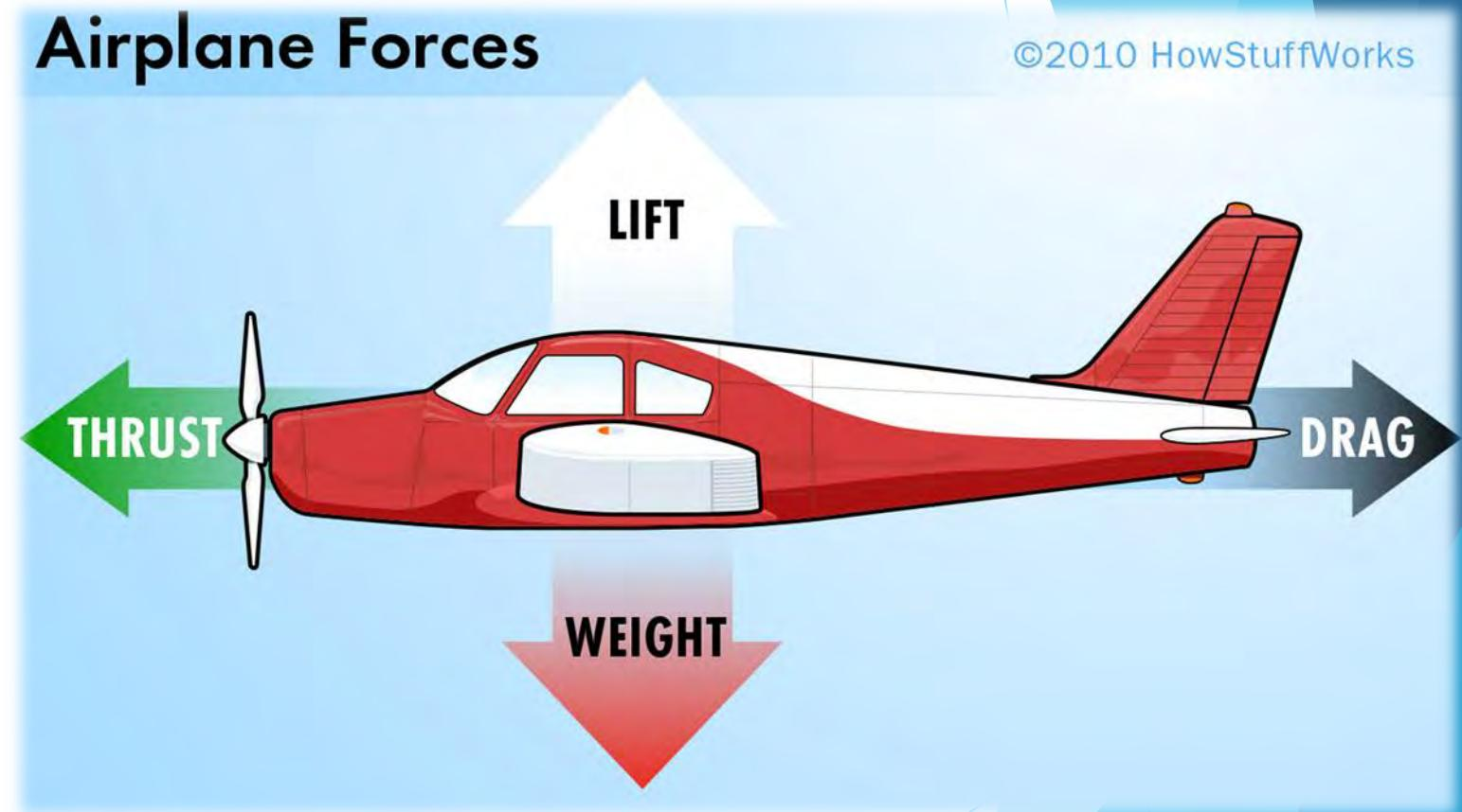
These four forces combined are what determine the flight characteristics of an aircraft.
