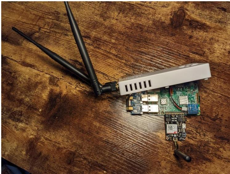
*Note.* The device is a Raspberry-Pi-based “Stratux” ADS-B receiver assembled by Crewdog Electronics that can receive both 978 MHz and 1,090 MHz ADS-B signals (hence the two long antennas). It is attached to a GSM device that gives the system the ability to communicate via cellular networks. A similar system with a LoRa instead of a GSM device can be used as the central computer.
