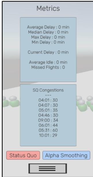
Figure 16 | Graphical user interface demonstrating metrics for delay and congestion in the simulation.
