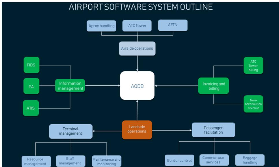
Figure 1 | The Airport Operational Database, which is commonly provided by IT groups like Leidos and Siemens, is the backbone of software in an airport (AltexSoft, 2020).
