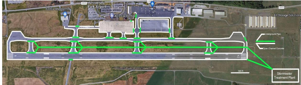
Figure 5: Estimated Location of STP and Concrete Open Channel at State College Airport
