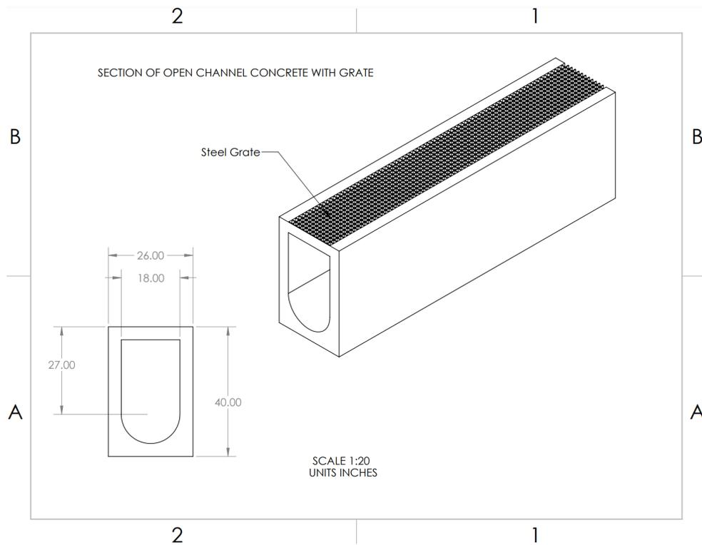
*Figure 6: Cross Section of Open Channel Concrete*
