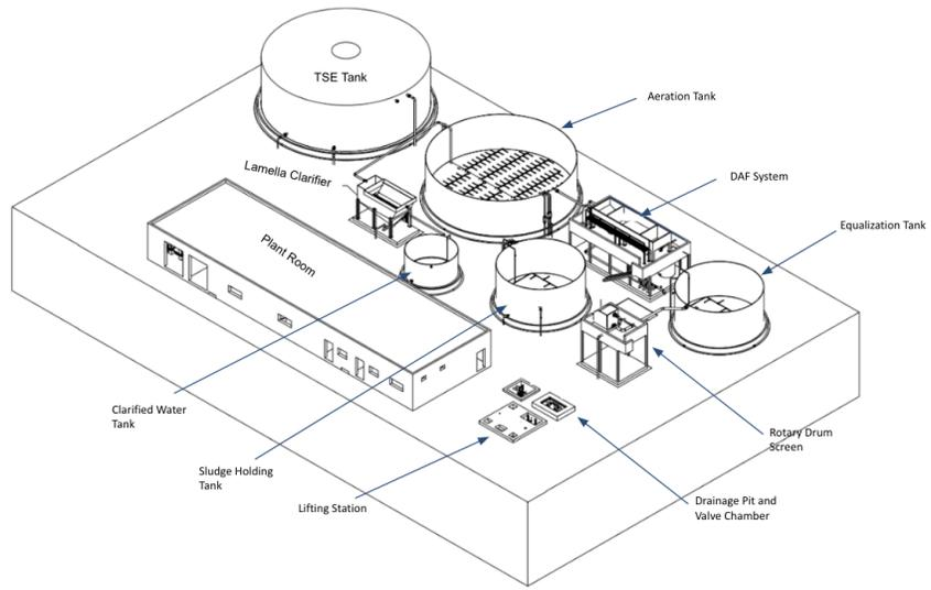
Figure 4: CAD Drawing of Stormwater Treatment Plant
