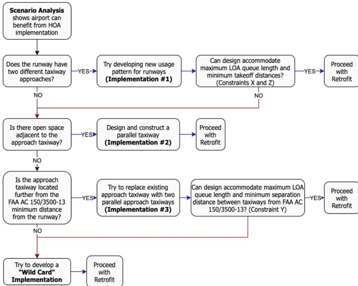
**Fig. 8.** Design and Construction Feasibility Workflow
