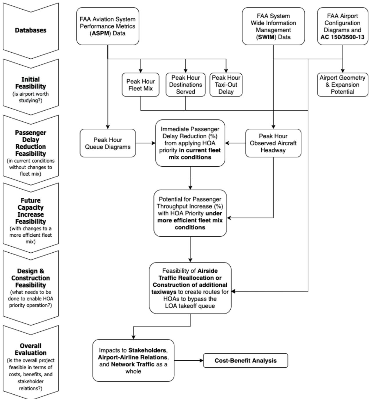
**Fig. 1.** Proposed Method for Evaluating Passenger Throughput Under HOA Conditions
