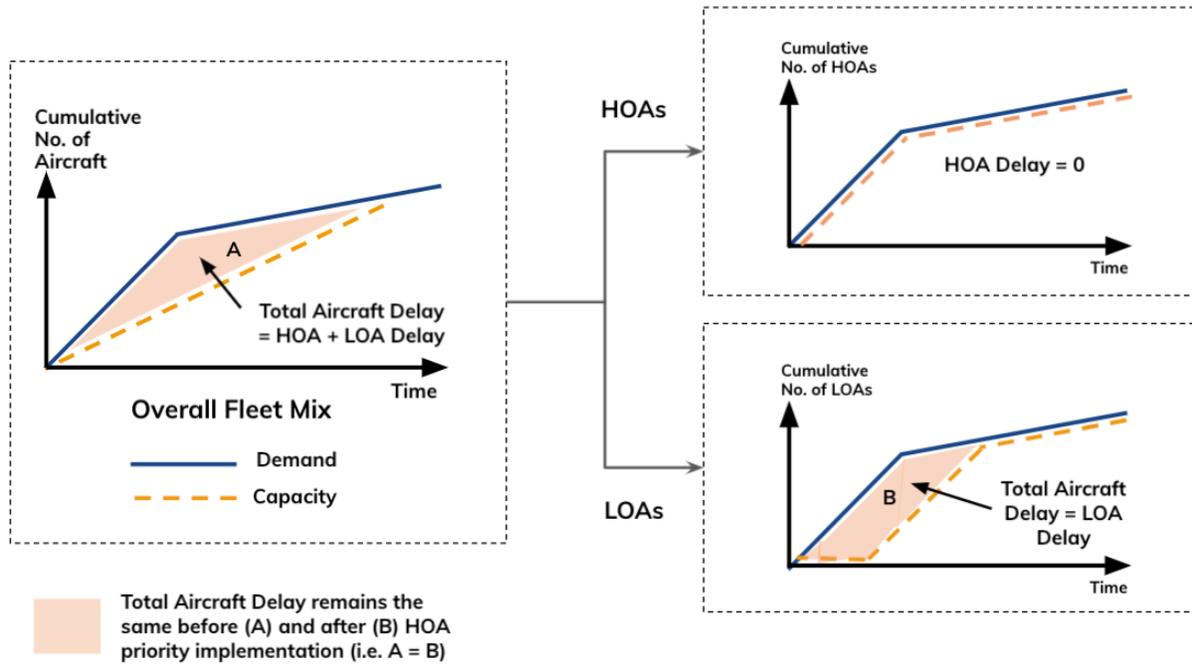
**Fig. 2.** Total Aircraft Delay is Transferred to LOAs under HOA Priority Regime
