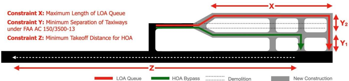
Fig.7. Splitting of Existing Approach Taxiway (Standard Implementation 3)
