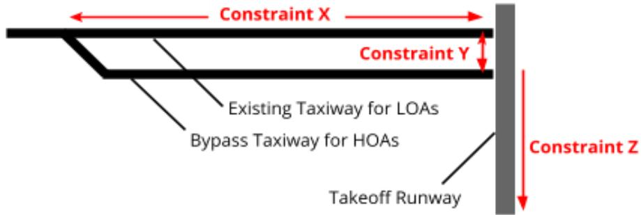
Fig. 5. Design and Constructability Constraints for HOA-Priority Taxiway Retrofits
