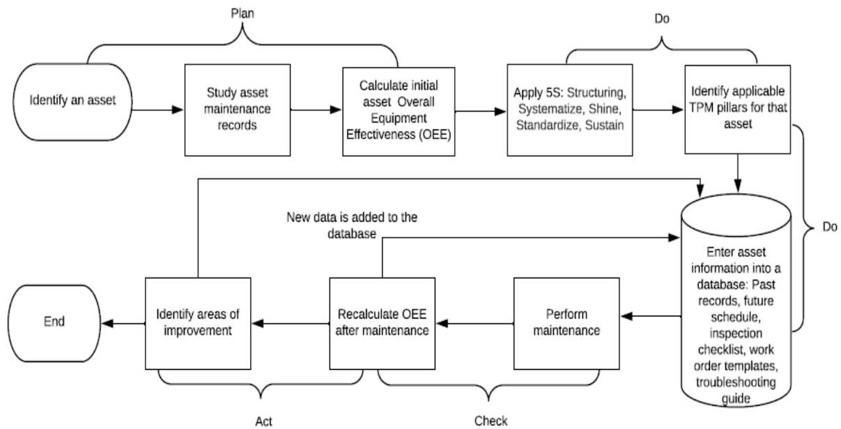
Figure 1. Process map developed by the team to show how TPM can be incorporated in the PDCA process approach
